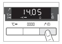
The Cook time  $\bowtie$  and End time  $\neg$  function indicators light up and the temperature is shown in the display. In this example, 200°C.
